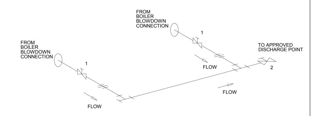
NOTE: WHEN SUPPLIED BY BRYAN UNIONS OTHER THAN SHOWN MAY BE USED WHERE NEEDED TO ALLOW REMOVAL OF PREPIPED ASSEMBLY FOR SHIPMENT.
