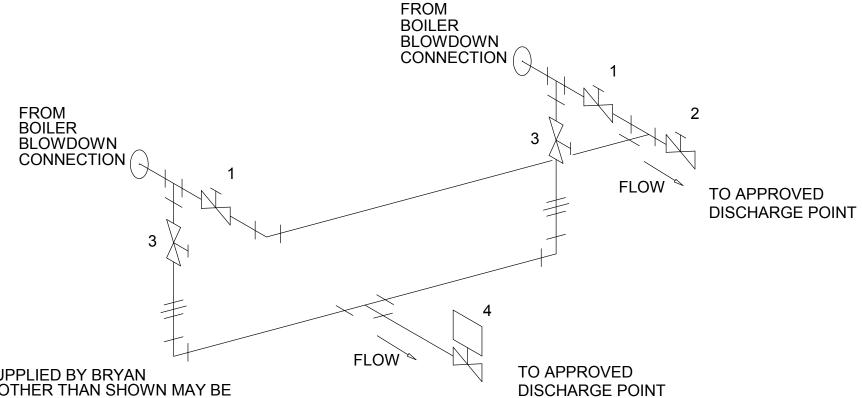
NOTE: WHEN SUPPLIED BY BRYAN UNIONS OTHER THAN SHOWN MAY BE USED WHERE NEEDED TO ALLOW REMOVAL OF PREPIPED ASSEMBLY FOR SHIPMENT.
