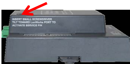
Figure 24 - LonWorks Service Pin Location
