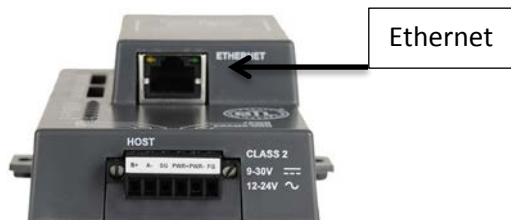
Figure 26 - ProtoNode Ethernet Port
