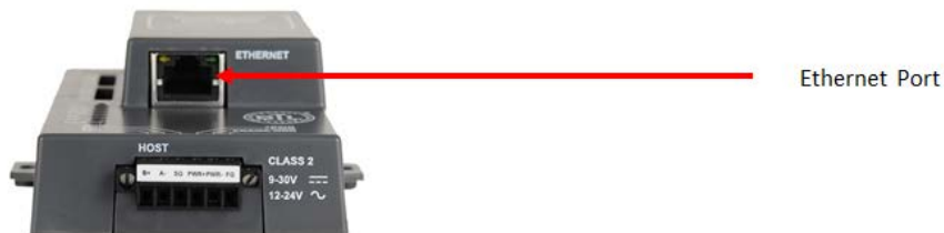
Figure 36 - Ethernet Port Location
