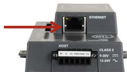
Figure 3 - Ethernet Connection on the ProtoNode
