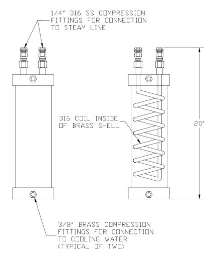
COIL PRESSURE - 1000 PSI MAX. SHELL PRESSURE - 1000 PSI MAX.
