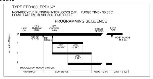
\*The EPD167 does not initiate a lockout if the M-D low fire start interlock remains open indefinitely during purge.
