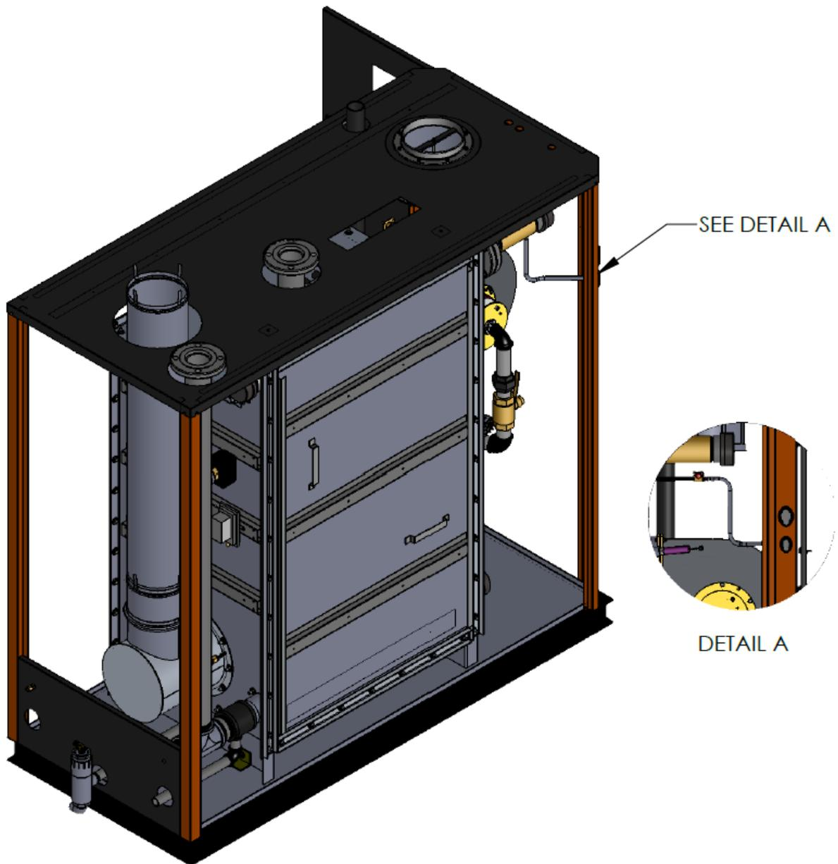
Add Stack piece to the stack transition. Add condensate trap to the condensate drain piping. Install temperature and pressure gauge in the latch post knockouts. Shown in detail A connect the flexible hose from the backside of the pressure gauge to the 1/4" ball valve. Connect the temperature probe from the gauge to the supply pipe.
