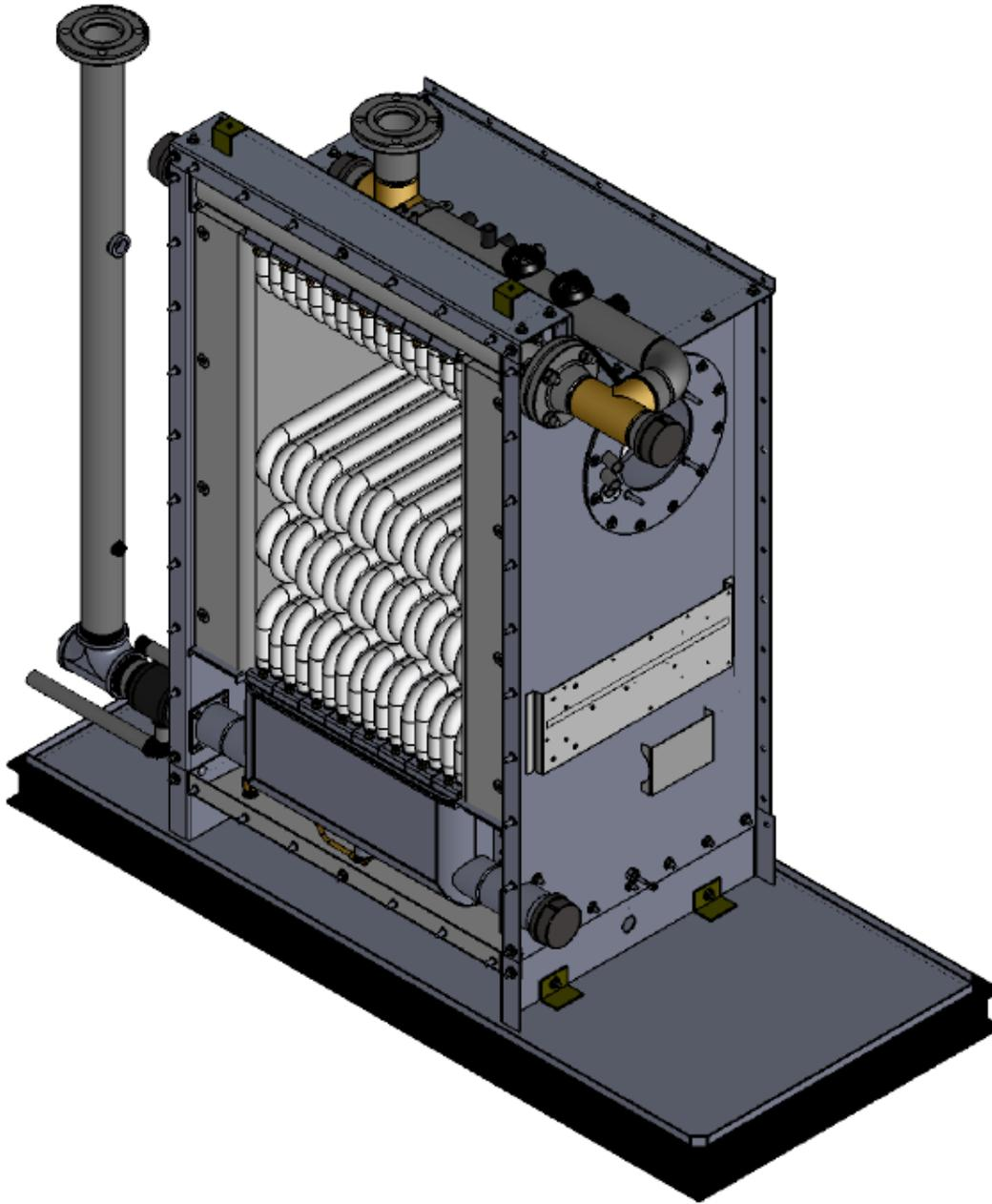
Insert all components that need to go into the supply piping. Plug all other holes not being used. Install and drive tubes. Step 1: Apply water to the boiler and inspect for leaks. Step 2: If there are leaks, shut off water and drain to relieve pressure to fix the leak. Repeat Steps 1 and 2 until there are no more leaks. Then, fasten all the tube clamps down on the top and bottom portions of the tubes.
