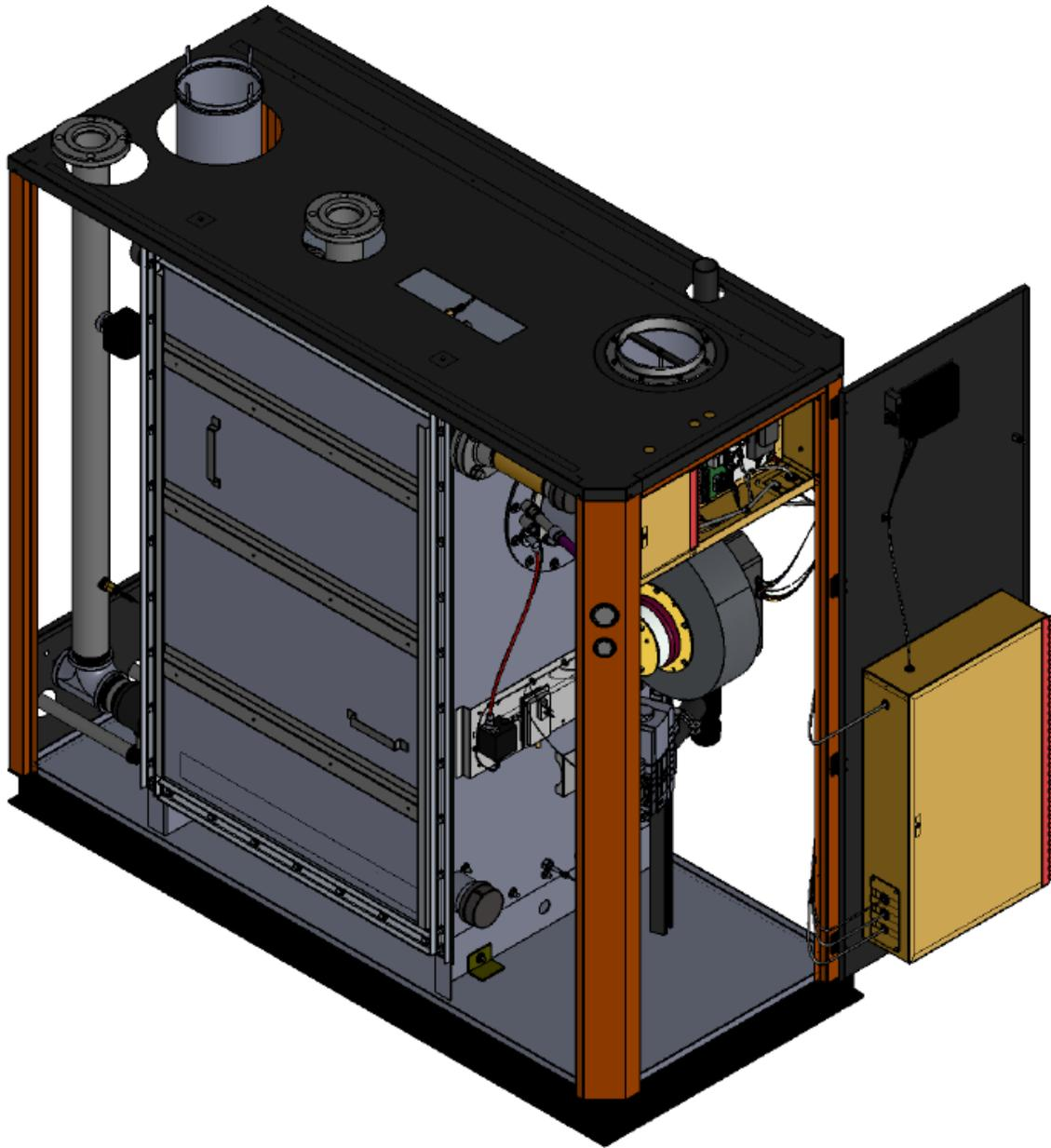
Wire up all components using the wire harnesses. Attach the ignitor cable from the spark generator to the ignitor. Once all the wiring is complete add control box patches for both the lower control panel and the upper control panel.
