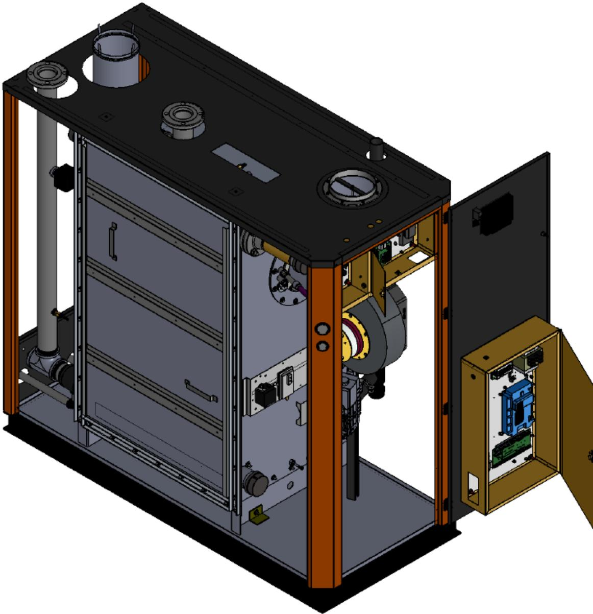
Level and mount the upper control box using the pilot holes on the post for the 1/2" self-tapping screws. On the lower control box, level the box and add 3/8" zinc washers and nuts to secure the box to the front door studs. Then place the wire insert panel on the studs and secure it with 3/8" zinc washer and zinc nuts.
