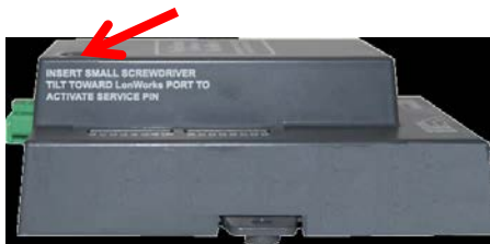
Figure 24 - LonWorks Service Pin Location
