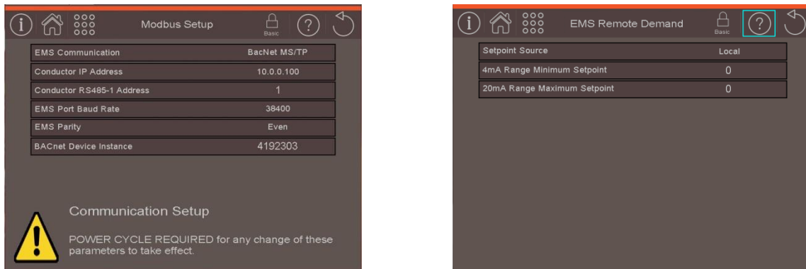
Figure 19: Modbus Setup Screens
